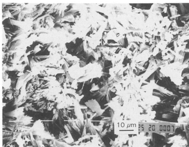
Figure 4 Scanning electron micrograph of the solid phases present in a partially reacted mixture of \beta -hemihydrate and water after 60 min (W/P ratio = 0.6).
